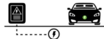
**EV Capable:** parking spaces that in addition to having EV ready requirements, also have conduit to a junction box or 240 volt-outlet that is ready for the installation of an EV charger
